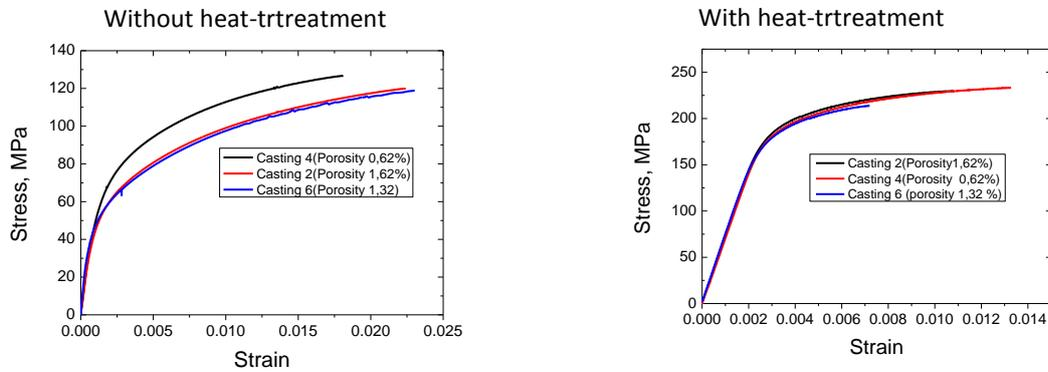
Tensile test experiments show that after heat treatment the strength significantly increases but ductility decreases, the stress-strain curves differ by failure strain
