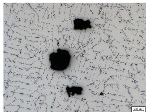
Both tomographical and metallographical surface characterization testifies to the existence of small pores (diameter around 20  $\mu\text{m}$ ) and big pores (200-400  $\mu\text{m}$ ).
