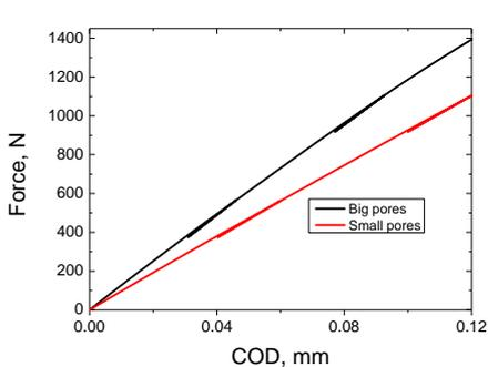
F-COD curve matching the instance of crack entering the cut-out of microstructure
