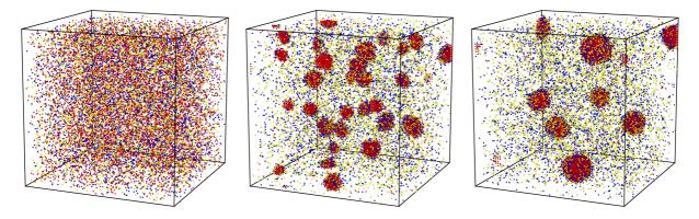
(a) T=500°C, t=0,  $\overline{R}$ =0 (b) t=8.8 hours,  $\overline{R}$ =1nm (c) t=79 hours,  $\overline{R}$ =1.57nm
